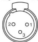
DMX - output XLR mounting-sockets (rear view):
