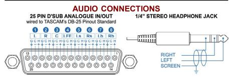
• **Interference:** If the unit is to be used where it maybe exposed to high levels of disturbance such as found close to a TV or radio transmitter, we advise that the unit is operated in a balanced configuration. The screens of the signal cables should be connected to the chassis connection on the XLR connector as opposed to connecting to pin1. The CMC7 conforms to the EMC standards.
